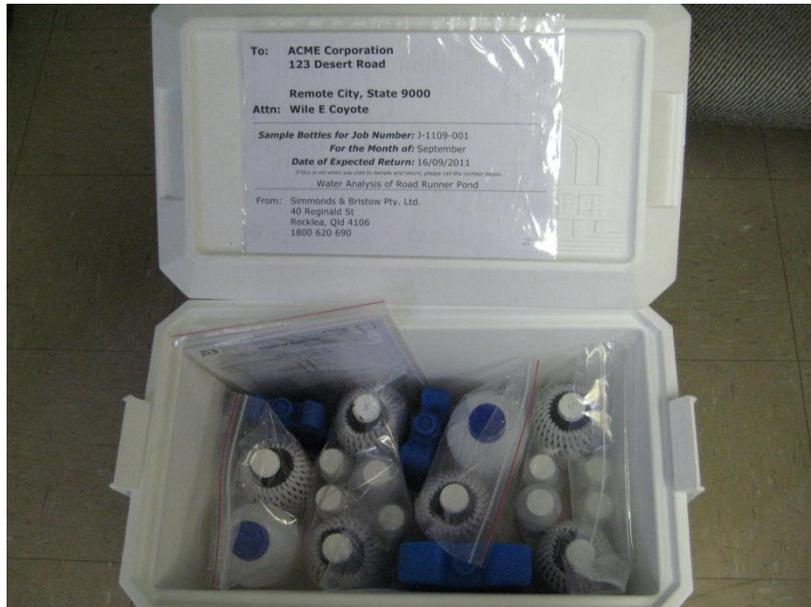
These bottles are prepared in compliance with AS2031 and Queensland Department of Environment Guideline and are colour coded accordingly.
