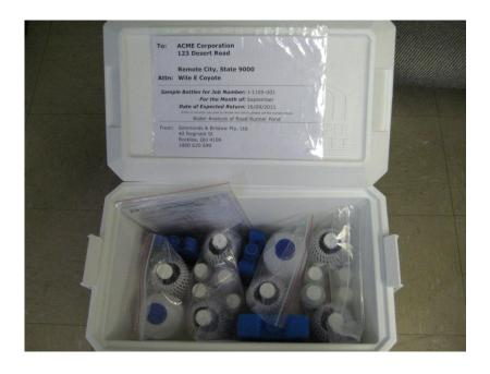
These bottles are prepared in compliance with AS2031 and Queensland Department of Environment Guideline and are colour coded accordingly.
